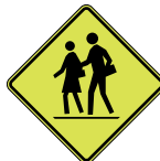
School crosswalk ahead
